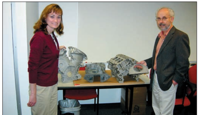
Figure 12. Magnesium powertrain components for the Duratec 2.5 L/V6 engine developed for the USCAR FreedomCAR program displayed by Joy A. Hines of Ford and Bob Powell of GM. 13
