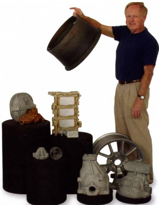
Figure 18. Earle Canavan holding a magnesium wheel preform above samples of other automotive magnesium parts made by the Magnesium Automotive Group.
