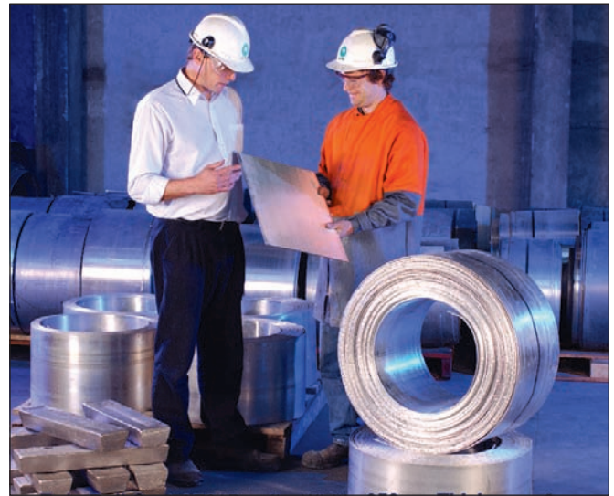
Figure 9. Twin-roll cast AZ31 coils of magnesium sheet (350 mm wide and 3 mm thick) being examined at CSIRO's pilot plant. 9
