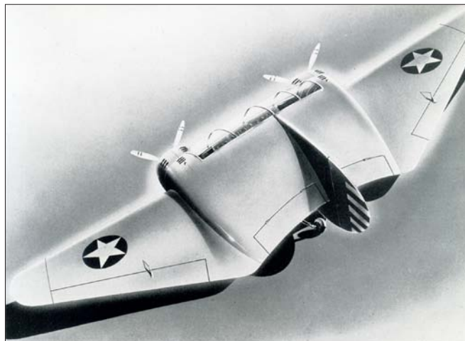
Figure 28. The magnesium intensive "Flying Wing" aircraft proposed during WWII. 47
