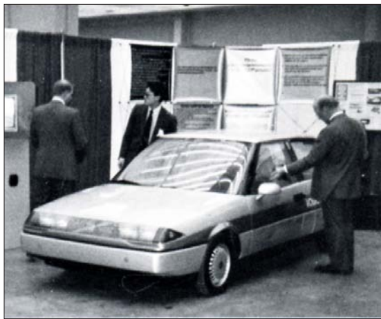
Figure 35. The experimental Volvo LCP 2000 at the 1985 SAE Congress had 7% of its body weight as magnesium castings that included a three-cylinder direct injected diesel engine block. 71
