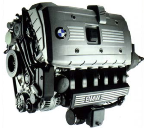
Figure 15. BMW NG6 engine (courtesy BMW AG). 20
