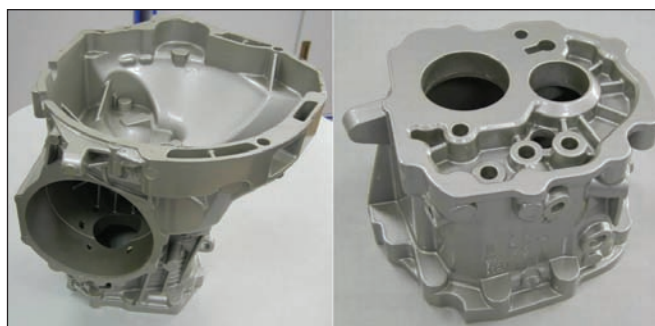
Figure 4. Magnesium gear box and cover for SAIC's Gol and Santana VW models. 6
