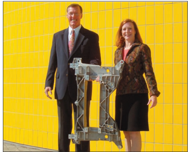
Figure 11. GM's Mike Meloeny and Lisabeth Riopelle (Hydro) showing the Corvette Z06 engine cradle that was high pressure die cast by Meridian Technologies from Hydro alloy AE44 at a 35% weight saving over the aluminum casting. 4
