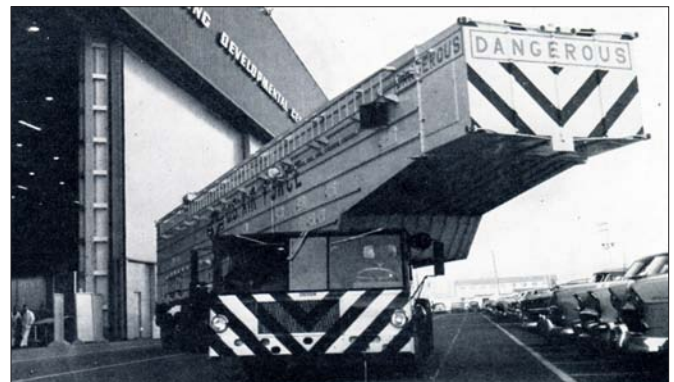
Figure 33. Magnesium was specified for doors and panels of the Minuteman missile shipping container in order to keep the shipment within highway load limits. 65
