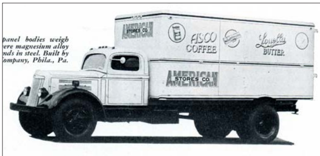
Figure 31. American Stores panel truck bodies of magnesium (supplied by Revere Copper and Brass Inc.) weighing 2100 pounds against 3600 pounds in steel. 61
