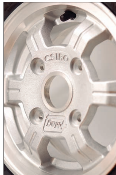
Figure 10. T-Mag cast magnesium wheel at CSIRO. 9
